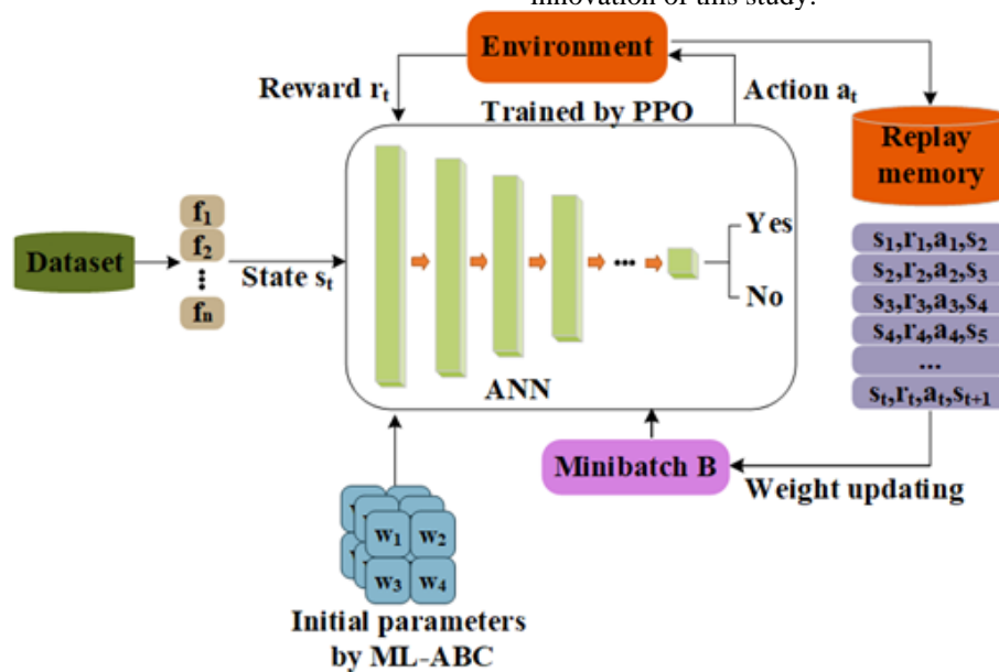
Figure 1: The proposed framework includes an ML-ABC for initial parameter setting and a PPO-based training for imbalanced classes.
