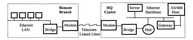
Figure 1: Network connections between a remote branch and the HQ of the bank
