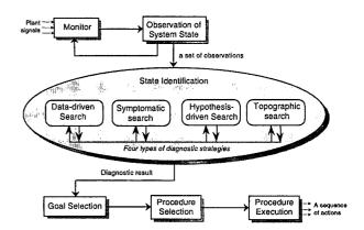
Figure 1: A schematic diagram of an operator's diagnostic and recovery tasks
