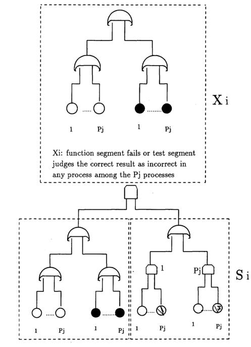
Xi: the ith version fails which activates the (i+1)th version. Si: in the (i+1)th version, the function segment fails and the test segment judgs the incorrect result as correct which causes the system failure.
