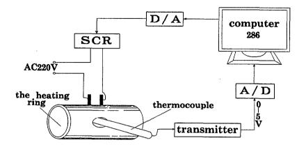
Figure 7: Fuzzy control system for temperature
