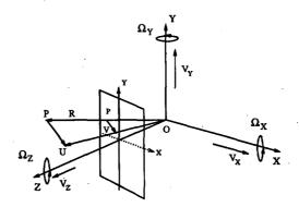
Figure 1: 3-D Formulation for Stationary Scene/Moving Viewer
