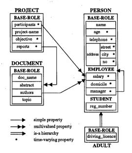
Figure 1: Example of ORM schema
