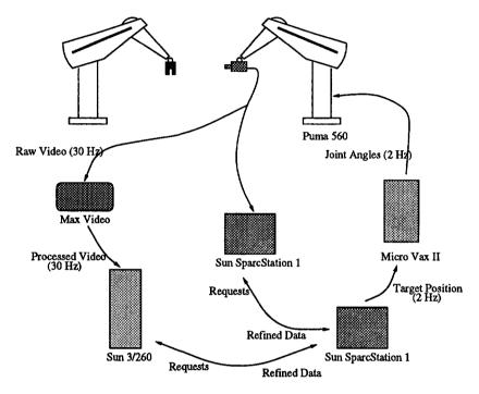
Figure 8: The Architecture of the System
