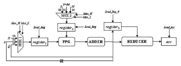
Figure 22: The modular multiplier architecture
