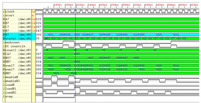
Figure 33: The modular multiplier behavior during the second multiplication: Montgomery(7,34,47) = 14
