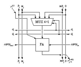
Figure 39: Basic PE architecture
