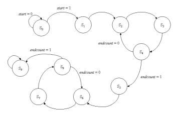
Figure 31: The state machine of the multiplier controller
