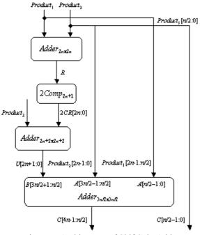
Figure 7: Architecture of ShiftSubnAdder<sub>2n</sub>
