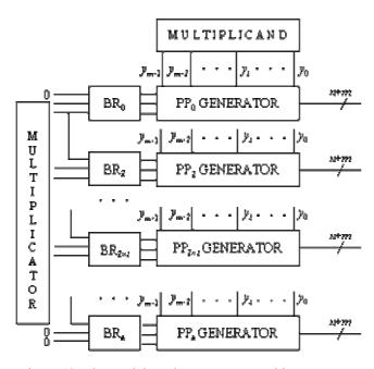
Figure 12: The partial product generator architecture.
