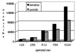
Figure 43: The *area×time* factor for iterative vs. systolic
