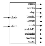
Figure 30. The interface of the multiplier controller
