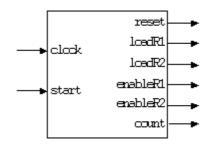
Figure 27: Interface of the Montgomery controller
