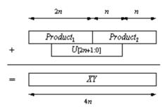
Figure 8: Last addition performed by ShiftSubnAdder<sub>2</sub>
