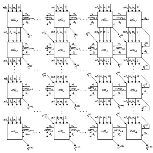
Figure 38: Systolic architecture of Montgomery multiplier
