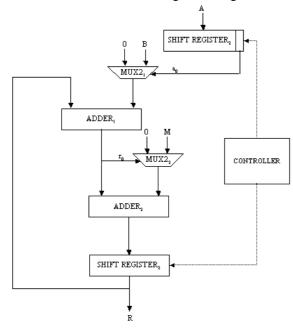
Figure 26: Montgomery multiplier architecture
