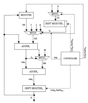
Figure 29: The modular multiplier architecture
