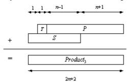
Figure 6: Operation performed by the ShiftnAdder<sub>2n</sub>
