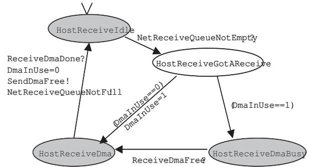
Figure 8: State transition diagram of the hostReceive module
