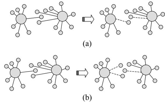
**Figure 4:** First Improvement Local Search procedures. (a) One movement of 1-interchange GAP local search. One client of the first cluster interchanges with a client from the other one (dotted lines). (b) One movement of 2-interchange GAP local search. One client of the first cluster interchanges with two clients from the other one (dotted lines).
