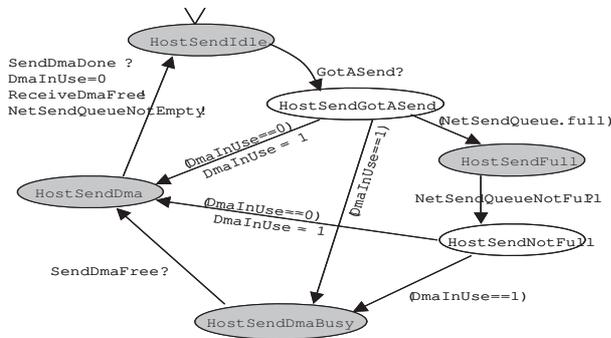
Figure 6: State transition diagram of the hostSend module
