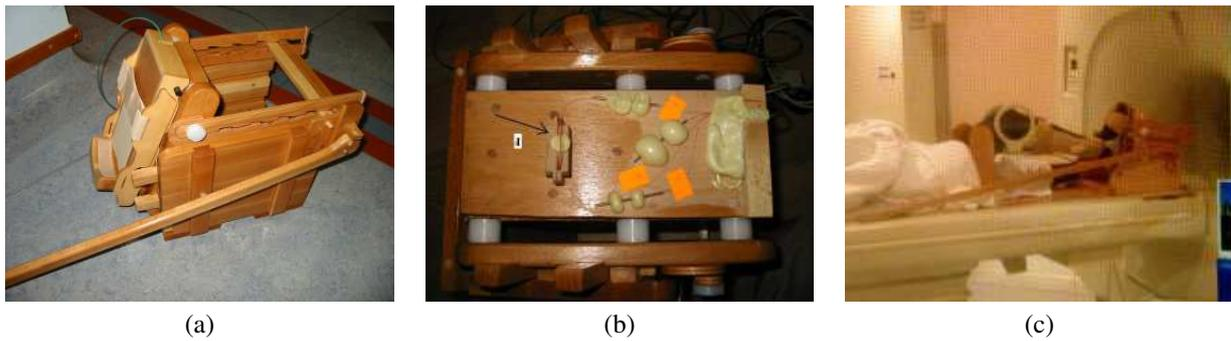
Figure 3: MR compliant exercise rig: a) wooden pedal, b) optical force sensor integrated on pedal, c) volunteer during additional parameter acquisition in the MR scanner.
