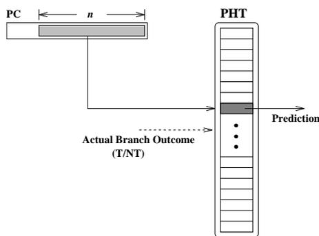
Figure 1: Implementation of Simple One-Level Branch Prediction
