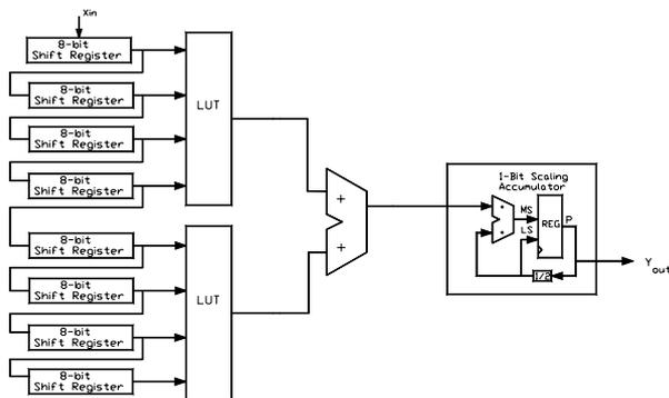
Fig. 4. A partitioned-LUT DA implementation of the Daubechies FIR filter.
