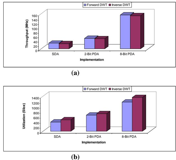
Fig. 9. Performance comparison (a). Throughput and (b). Utilization.
