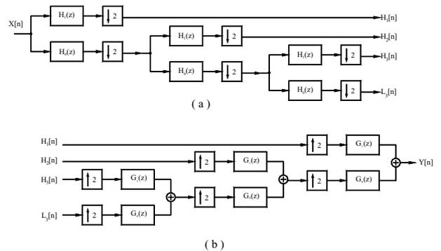
Fig. 2. Mallat's quadratic mirror filter tree used to compute the coefficients of the (a). forward and (b). inverse wavelet transforms.
