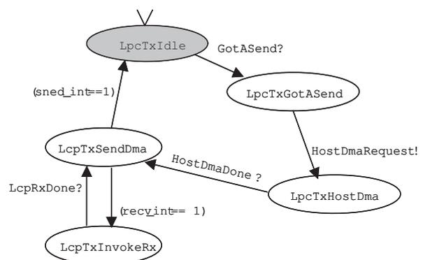
Figure 5: State transition diagram of the lcpTx module
