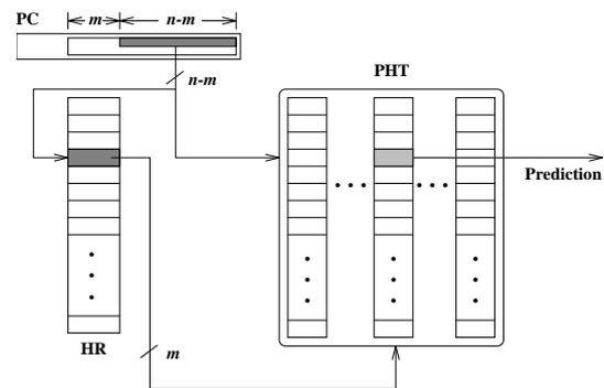
Figure 2: Implementation of Per-Address Correlation-based Branch Prediction
