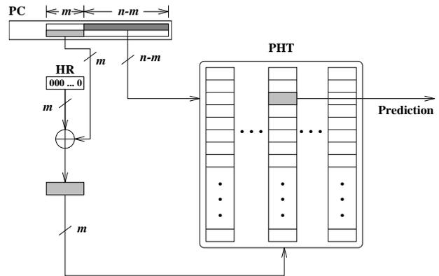
Figure 6: One-Level Predictor as A Special Case
