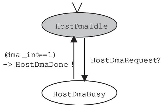
Figure 4: State transition diagram of the hostDma module
