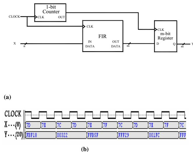
Fig. 7. (a). Implementation and (b). functional simulation of the decimator.
