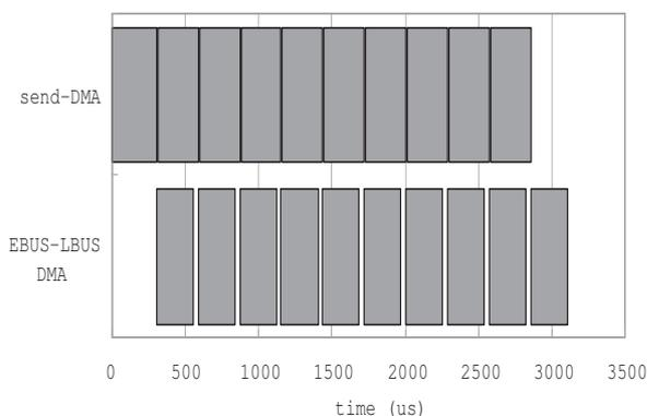
Figure 11: DMA overheads of MCP
