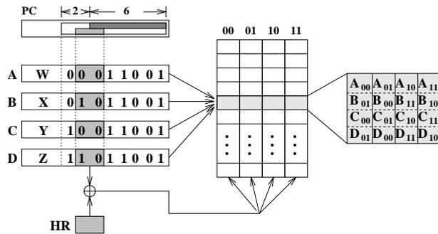
Figure 12: A Hybrid Design of Two-Level and Gshare Predictors
