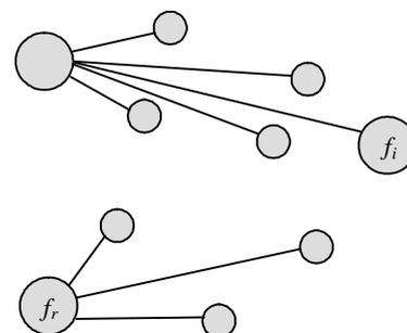
**Figure 1:** Overview of the local search procedure. Solid lines connect clients to medians,  $f_i$  is the candidate to enter the solution as a median, and  $f_r$  is the median that will leave the solution.
