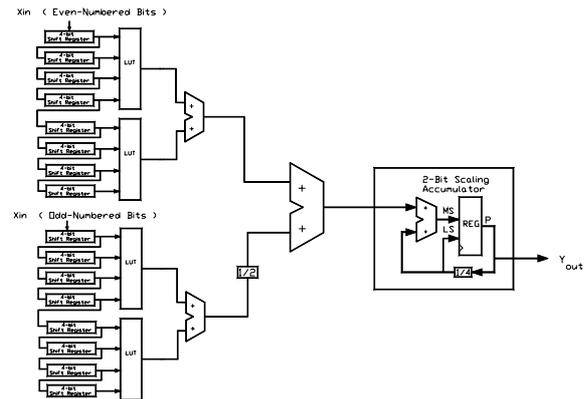
Fig. 5. A 2-bit PDA Daubechies FIR filter.
