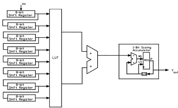
Fig. 3. A DA implementation of the Daubechies FIR filter.
