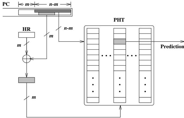
Figure 7: Two-Level Predictor as A Special Case
