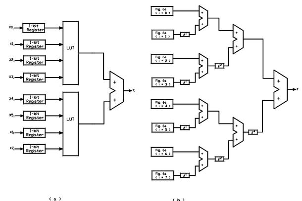
Fig. 6. (a). A single-bit and (b). an 8-bit PDA Daubechies FIR filter.
