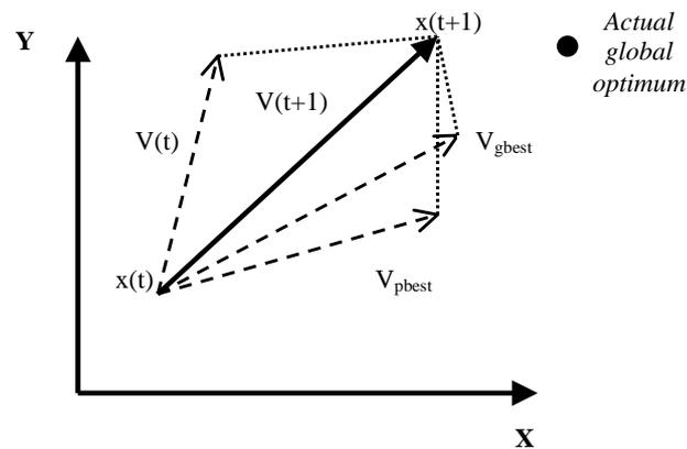
Figure 1: A representation of the particle position-update process.
