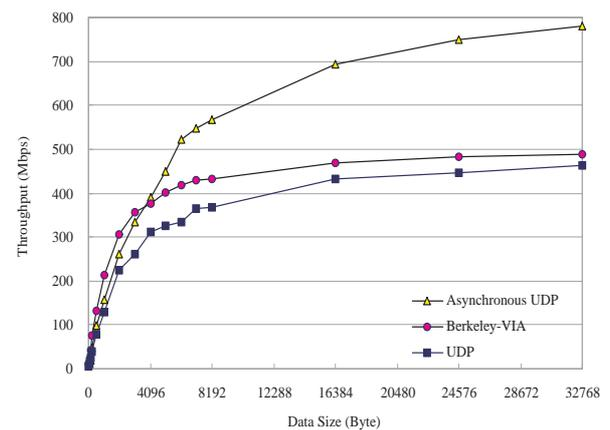
Figure 1: Throughput comparison of Asynchronous UDP, Berkeley-VIA, and UDP
