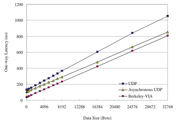
Figure 2: One-way latency comparison of Asynchronous UDP, Berkeley-VIA, and UDP
