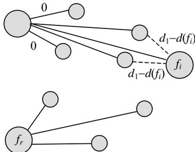
**Figure 2:** First term of the right hand side of Eq. (11). Clients not allocated to  $f_r$  that will profit from the insertion of  $f_i$ . Solid lines connect each client to a median, dotted lines represent the new connections,  $f_i$  is the candidate to enter the solution as a median, and  $f_r$  is the median that will leave the solution.
