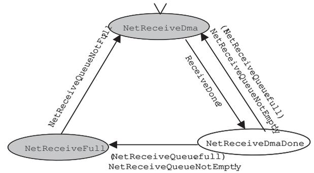
Figure 9: State transition diagram of the netReceive module
