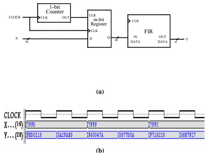
Fig. 8. (a). Implementation and (b). unctional simulation of the interpolator.
