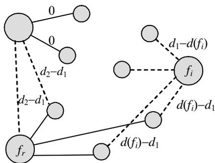
**Figure 3:** Second term of the right hand side of Eq. (11). Clients allocated to  $f_r$  that will profit or not from the exit of  $f_r$ . Solid lines connect each client to a median, dotted lines represent the new connections,  $f_i$  is the candidate to enter the solution as a median, and  $f_r$  is the median that will leave the solution.
