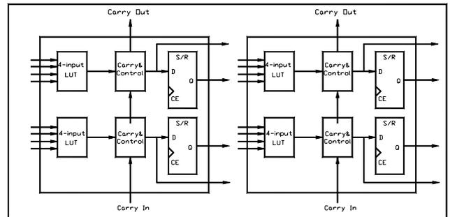
Fig. 1. Simplified Architecture of Virtex configurable logic block.
