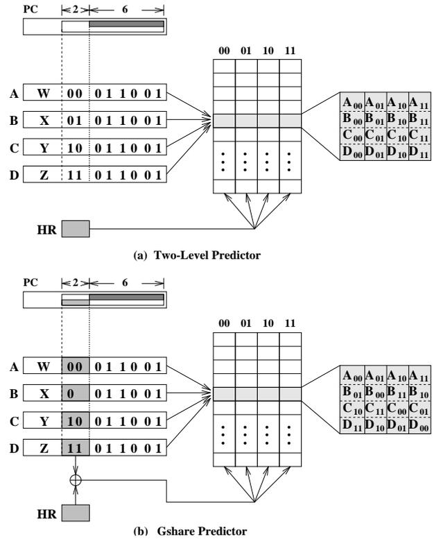
Figure 11: Difference between Gshare Predictor and Two-Level Predictor
