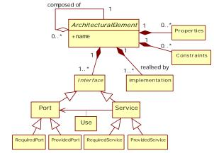
Figure 2: Structure of an architectural element in C3.
