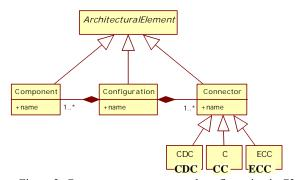
Figure 3: Component, connector, and configuration in C3.
