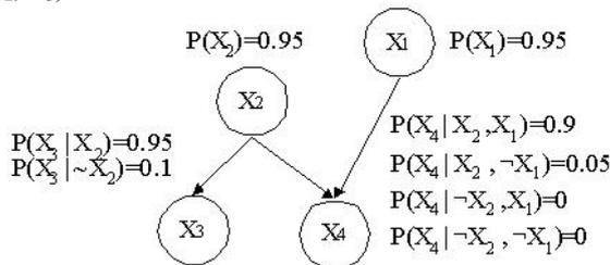
Figure 6. The structure of a Bayes Network
