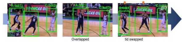
Figure 14: Boxes that are temporarily unrecognized are assigned new tracking IDs.
