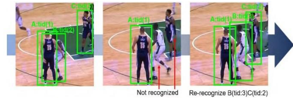
Figure 13: The tracking IDs of two overlapping player boxes are mistakenly swapped.
