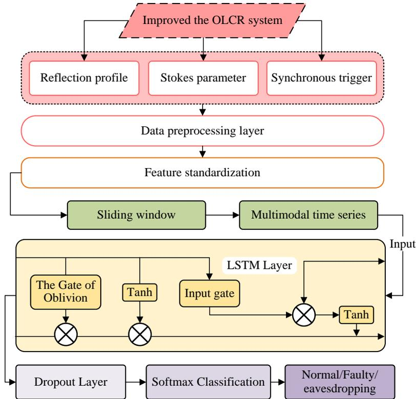
Figure 6: Intelligent intrusion recognition method combining polarization state angular velocity and LSTM.
