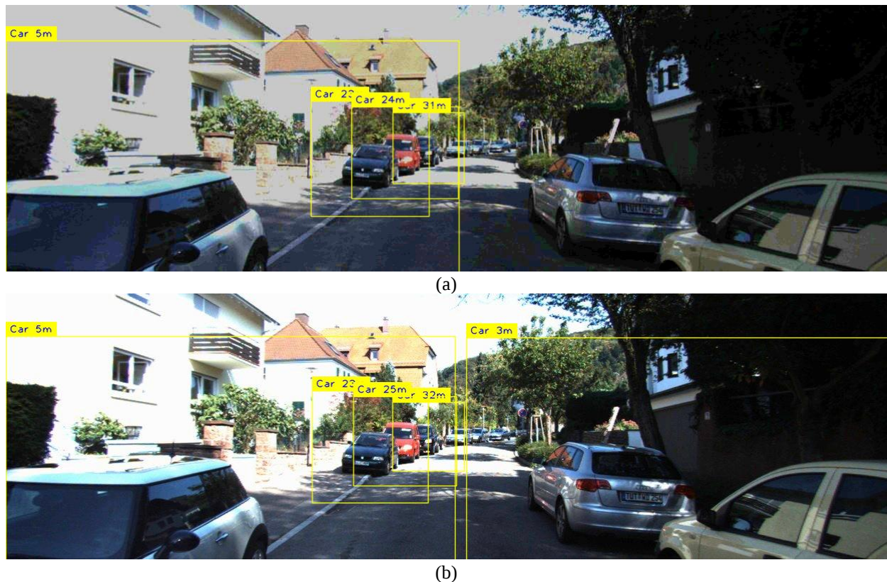
Figure 13: (a) Results of increased light intensity, object prediction, and distance prediction in the 4 th sample. (b) Results of increasing light intensity, object prediction, and distance prediction on the 17 th sample
