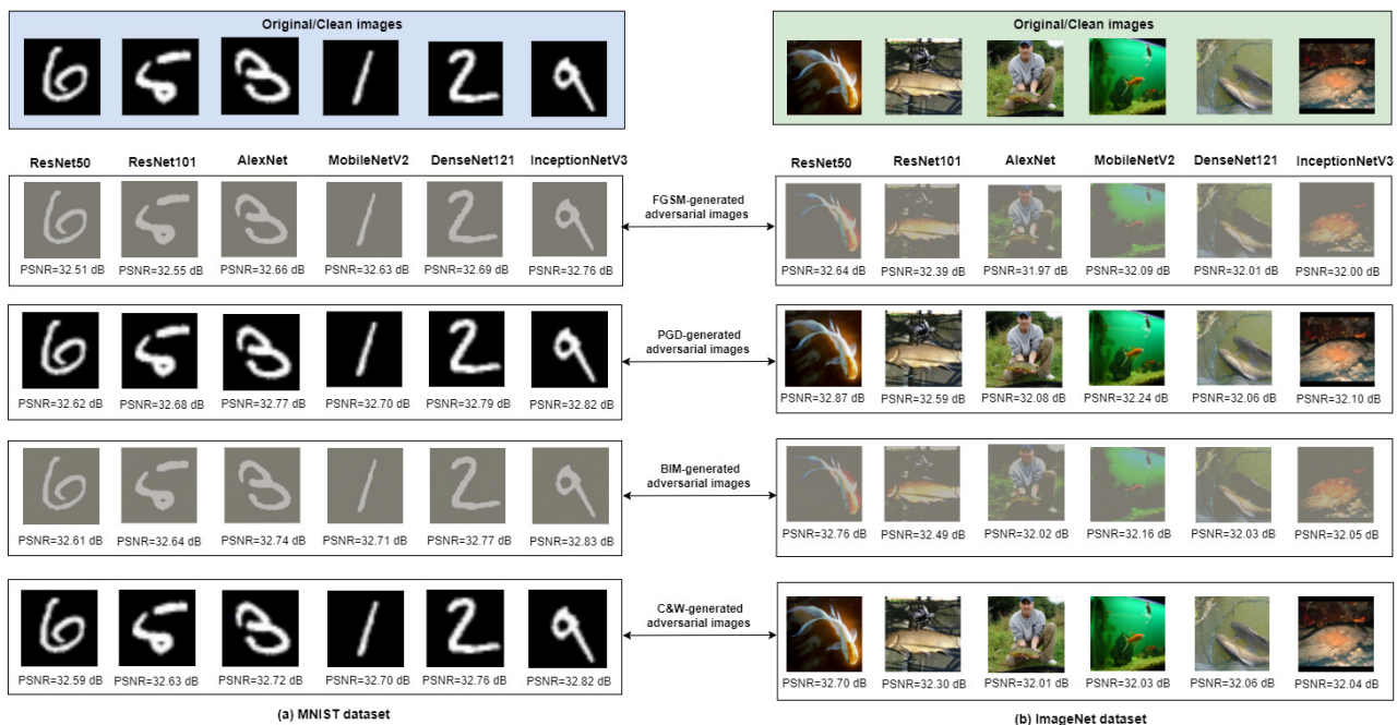
Figure 1: Visualization of adversarial examples generated by four attack methods (FGSM, PGD, BIM, and C&W) across six CNN architectures (ResNet50, ResNet101, AlexNet, MobileNetV2, DenseNet121, InceptionNetV3). Subfigure (a) shows results on the MNIST dataset, while subfigure (b) shows results on ImageNet dataset. The top row in each subfigure contains original (clean) images, while the rows below show adversarial versions organized by attack method and model. Peak Signal-to-Noise Ratio (PSNR) values, indicating the similarity between adversarial and clean images, are shown beneath each adversarial image.
