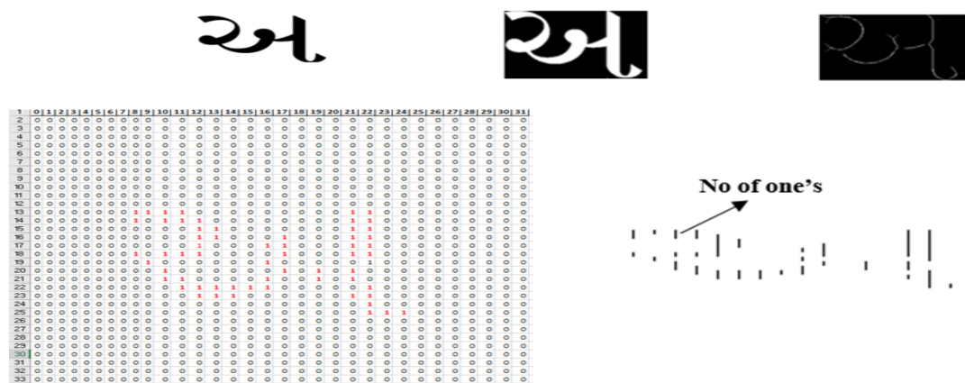
Figure 8: (a) Input Image (b) Preprocessed Image (c) Thin Boundary Extraction of image (d) Char array with 0's and 1's value (e) Text Shape of Gujarati text 'A' (See the results from left to right)
