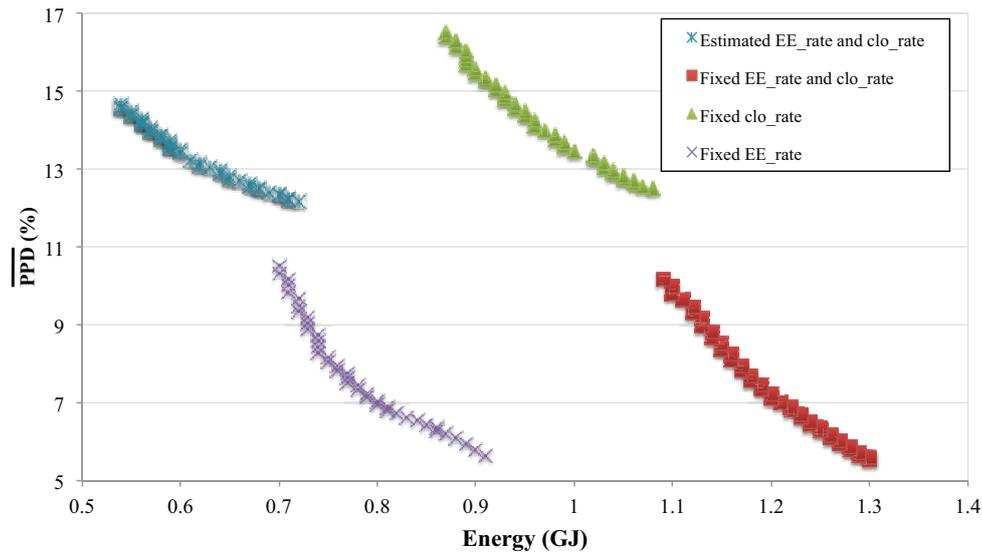
Figure 5: Comfort/consumption plane: The X axis represents the energy in GJ, consumed by HVAC; the Y axis represent the comfort experience -  $\overline{PPD}$ , expressed in %. Each marker presents a result of a simulation run for different  $PMV_{ref}$  and for a different assumption of the occupant's parameters configuration
