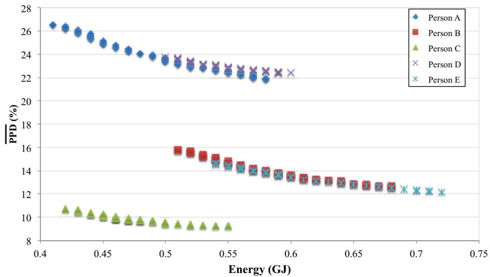
Figure 4: Comfort/consumption plane: the X axis represents the energy in GJ, consumed by HVAC; the Y axis represents the comfort experience -  $\overline{PPD}$ , expressed in %. Each marker presents a result of a simulation run for different  $PMV_{ref}$  and for different person
