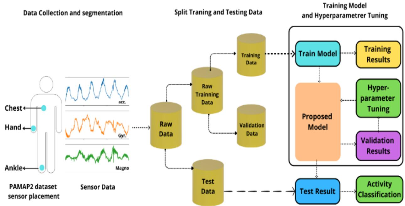
Figure 1: The schematic diagram of the proposed LSTM-Based model for sensor-based HAR
