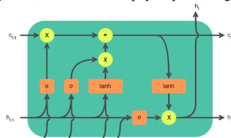
Figure.3. The Internal Structure of The LSTM Cell[31]
