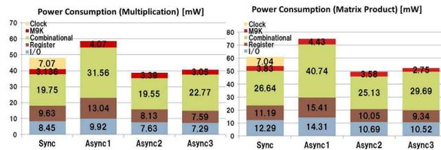
Figure 19: Dynamic power consumption of MIPS processors: (a) multiplication and (b) matrix multiplication.
