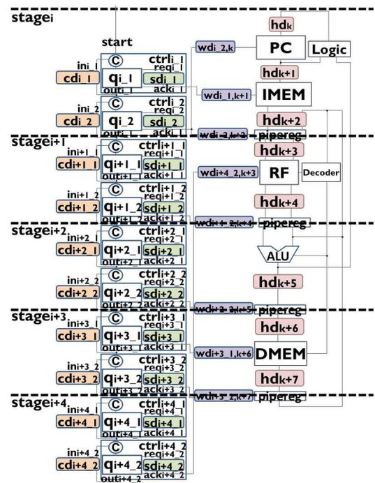
Figure 2: An asynchronous processor model with bundled-data implementation.
