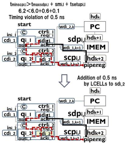
Figure 15: Delay adjustment for a setup constraint.
