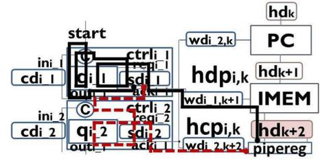
Figure 4: Data-path  $hdp_{i,k}$  and control path  $hcp_{i,k}$  for a hold constraint.
