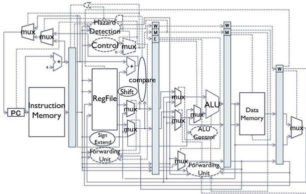
Figure 16: Block diagram of the MIPS processor in [12].
