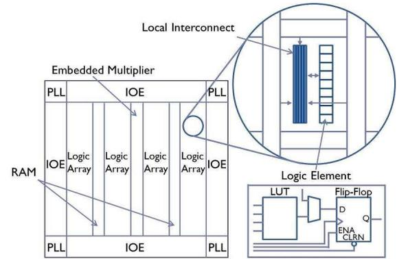
Figure 7: Structure of Altera Cyclone IV FPGA [10].
