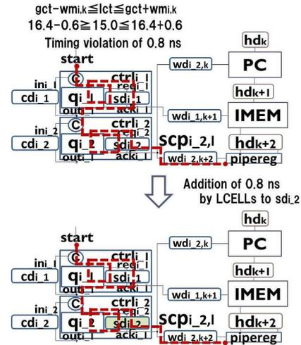
Figure 14: Delay adjustment for simultaneous writing constraints.
