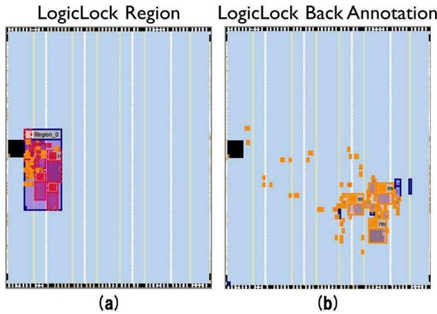
Figure 13: Effect of placement constraints: (a) based on a region and (b) based on the back annotation.
