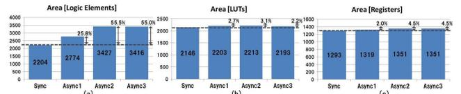
Figure 17: Area of MIPS processors: (a) the number of LEs, (b) the number of LUTs, and (c) the number of registers (DFFs).
