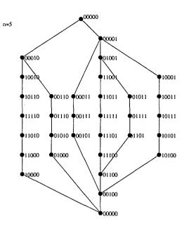
Figure 7: The communication scheme for 5-cube
