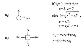
Input or output (c, s) of QR decomposition will be treated as y in the following sections.
