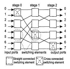
Figure 1: Multistage Interconnection Network (MIN)
