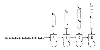
Figure 12: Data inputs in horizontal array
