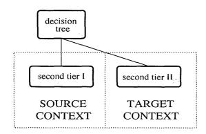
Figure 1: The decision tree with a second tier is transferred from the source context into the target context. The adaptation is carried out by re-induction of the second tier without the need to change the tree.
