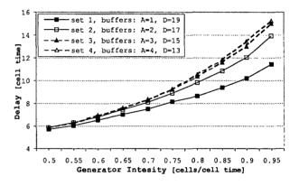
Figure 16: Mean Cell Delay of cell type D
