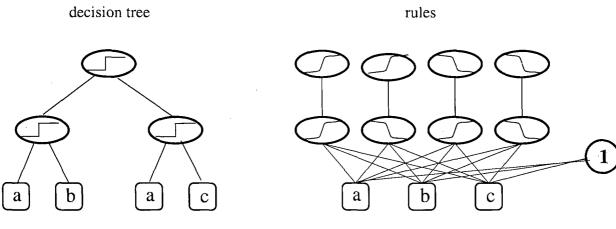
Figure 2: The decision tree is interpreted as a set of rules with "soft" tests. The second tier weighs the impact that each rule has on the individual concept labels.
