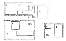
Figure 2: Planar view of an R-tree.
