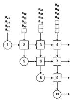
Figure 1: Triangular systolic array (n=4)
