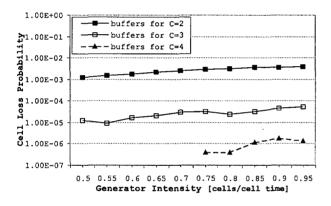
Figure 14: Cell Loss Probability for the CBR traffic class
