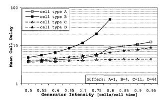
Figure 10: Mean Cell Delay for Set 1
