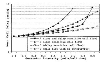
Figure 7: Mean Cell Delay for cell types, while buffer size for each cell type is 10
