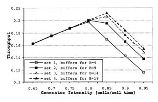
Figure 13: Throughput if cell type B for set 1-4
