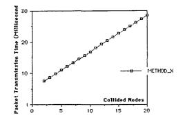
Fig. 9. Worst Case Time to Transmit (METHOD\_X)
